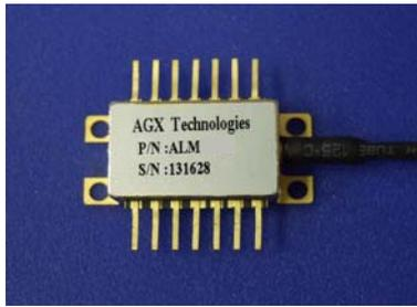
The ALM5Q series of 1550nm DFB laser modules are intended for use in the transmission of broadband analog signals. Their high linearity makes them especially suitable for CATV broadcast and narrowcast applications. All critical components, including optical isolator, TEC, thermistor, laser, and monitor photodiode are hermetically sealed in a butterfly package.
