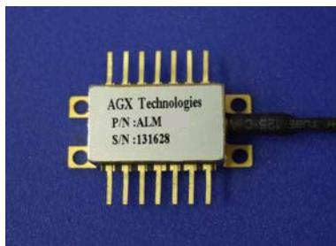
The ALM5R series of 1550nm DFB laser modules are intended for use in the transmission of broadband analog signals. Their high linearity makes them especially suitable for CATV return and narrowcast applications. All critical components, including optical isolator, TEC, thermistor, laser, and monitor photodiode are hermetically sealed in a butterfly package.
